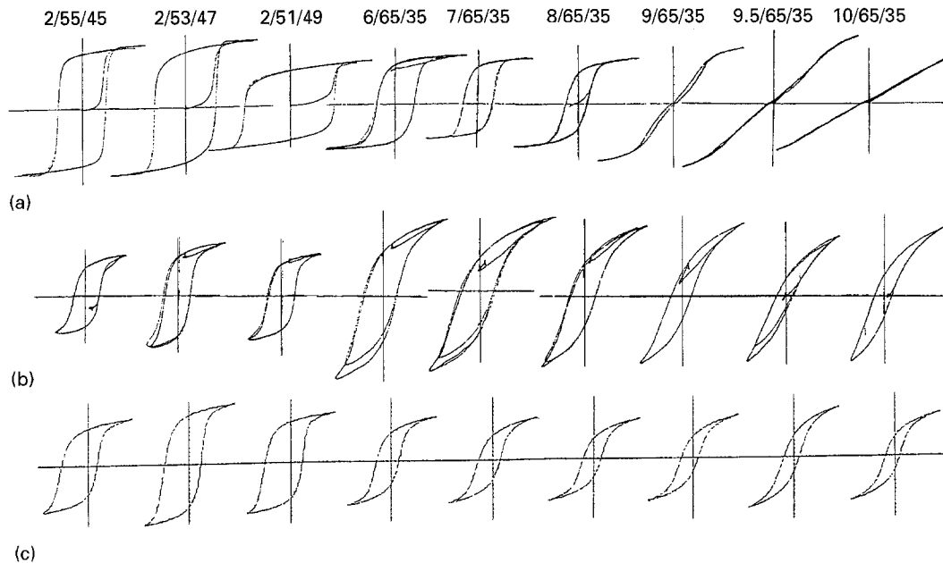
Figure 1 Polarization versus electric field hysteresis loops of PLZT bulk ceramics and thin films on silver. (a) Bulk ceramics, a.c.; (b) thin films, d.c.; (c) thin films, a.c.
